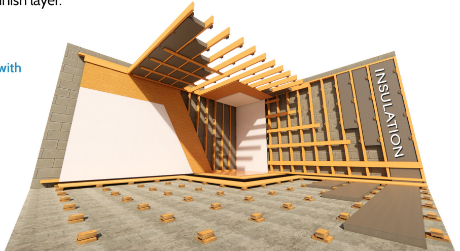
Fig. 1 Studio Float IsoRaft Deck Rafts on concrete slab with insulation in between IsoRafts, Walls showing insulation between studs with IsoRafts 16" OC horizontally and 24" OC vertically. Furring strips are attached to the IsoRafts and plywood, sheetrock or other sheathing materials attached to furring strips. Ceiling follows same application as walls.
